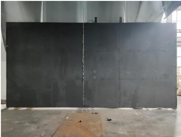
Rear view - TC Location of side wall. From the bottom to up, TCs were RW-1 to RW-24
