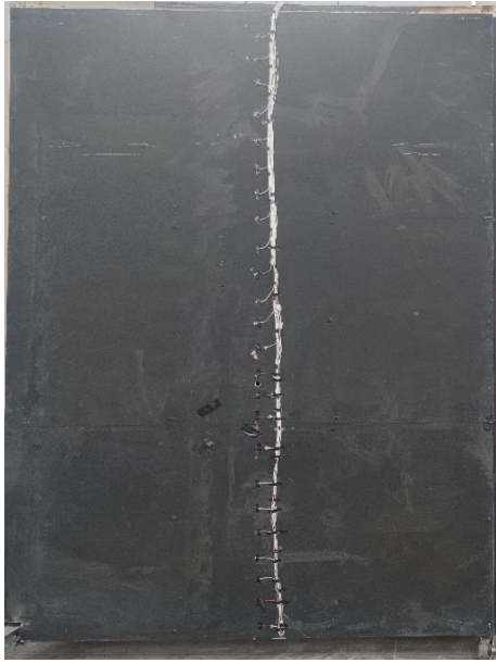
Front view - TC Location of front wall. From the bottom to up, TCs were FW-1 to FW-24
