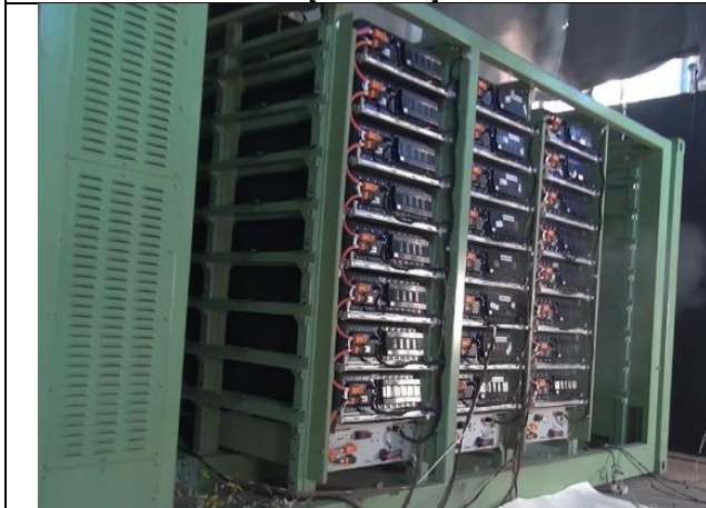
(c) Initiating cell 20-2 Thermal runaway [00:41:48]
